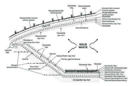
Fig. 1 – Solid Waste Containment System (Cover and Liner) with High Geosynthetic Utilization; Koerner (2005)
