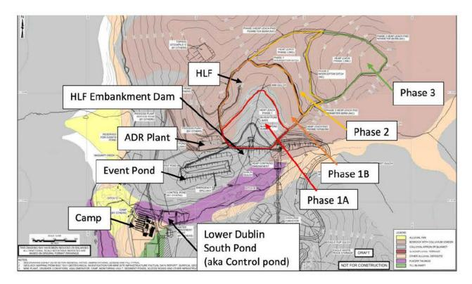
Figure 1: Layout plan of mine facilities near the HLF (extracted from drawing EGHLF-XD-01-03 in 2017 design report for HLF Phase 1A by BGC Engineering Inc. (BGC) (BGC, 2018))
