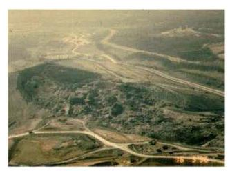
(a) Multiple rotational failure (500,000 m<sup>3</sup>)
