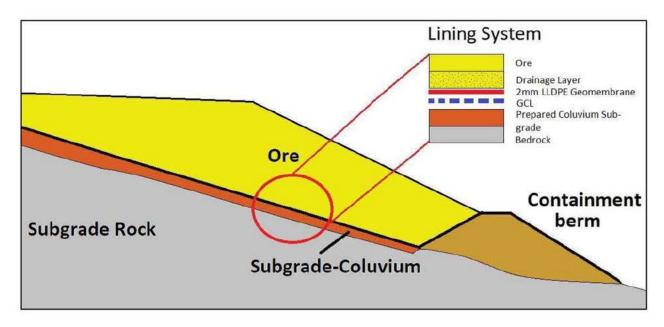
Figure 24: Overview of HLF component parts considered for analysis.
