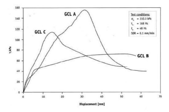
(a) Reinforced GCLs; "A" (needle punched), "B" (stitch bonded), and "C" (thermally locked)
