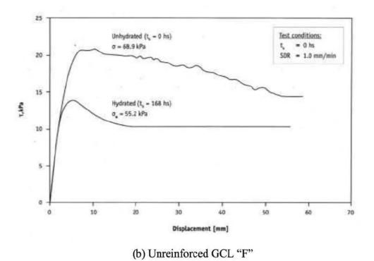
Fig. 7 – Shear Stress Versus Displacement Curves for Different Reinforced and Unreinforced GCLs; Zornberg, et al. (2005)
