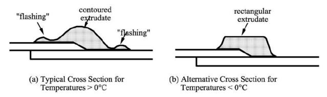
Figure 1 - Extrusion Fillet Patterns
