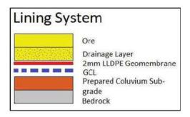
Figure 2: Graphical Representation of the lining system
